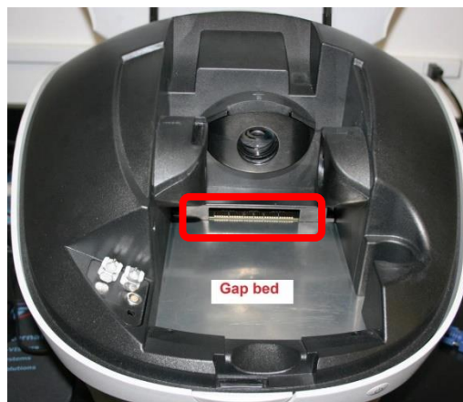
These contacts fit into a socket with complementary contacts in the back of the sample compartment gap-bed.
